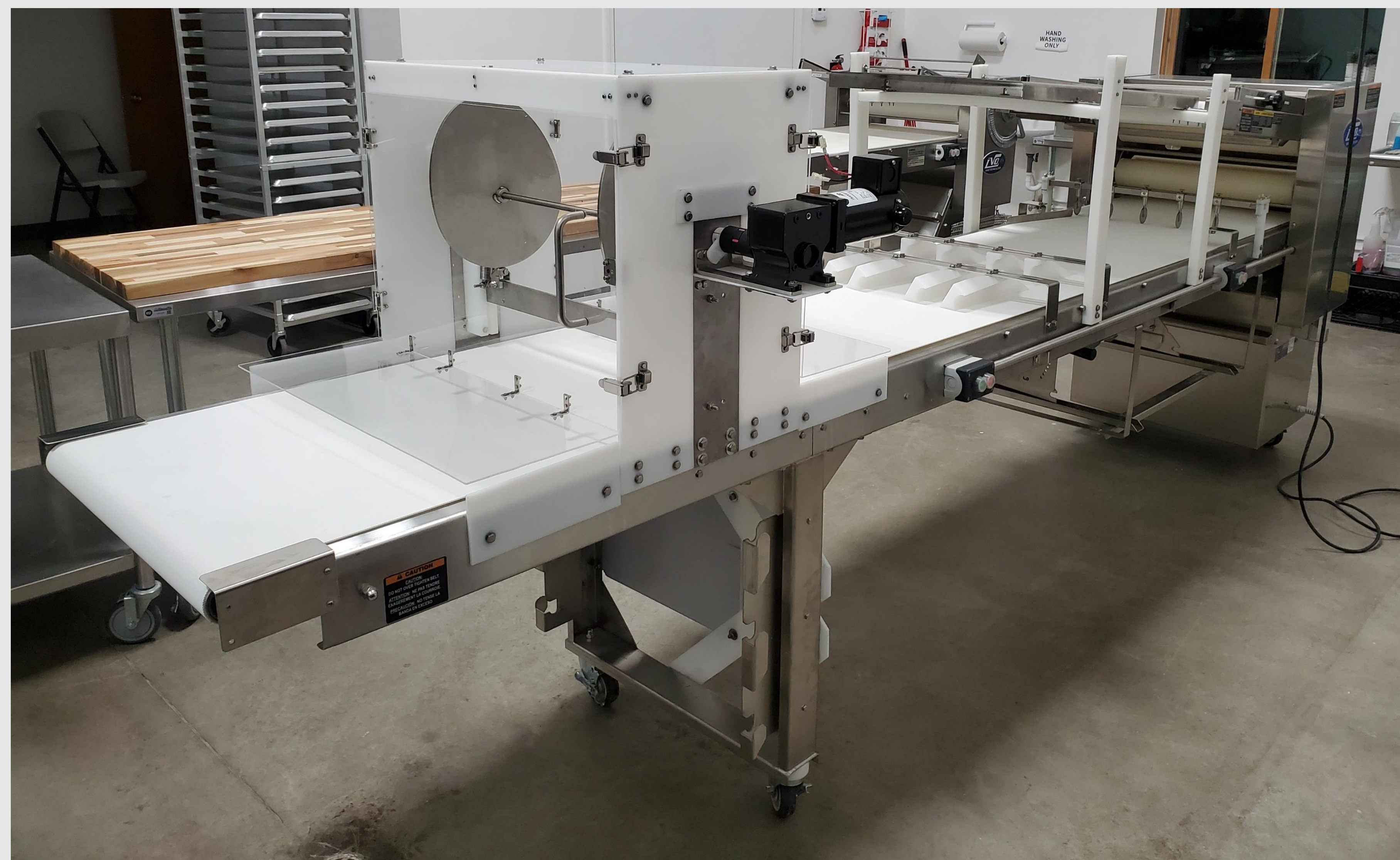
Figure 4. Integrated conveyor system
